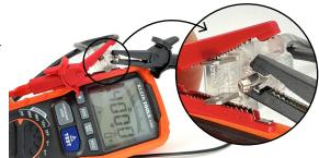
Notes: Set megger to 1000v. Both prongs of plug need to be shorted together during test, as shown above.
