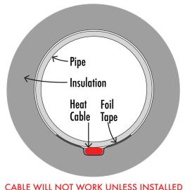
CABLE WILL NOT WORK UNLESS INSTALLED DIRECTLY ON PIPE AND INSULATED AS SHOWN
